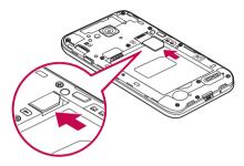
3 Insert the battery into place by aligning the gold contacts on the phone and the battery (1) and pressing it down until it clicks into place (2).
