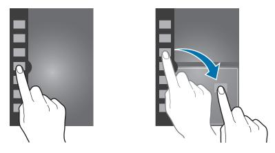
Drag the bar between the application panels up or down to adjust the size of the panels.
